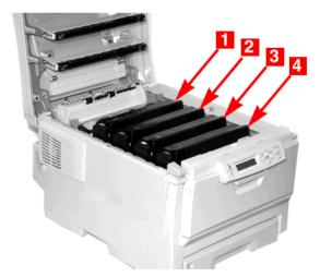
3. Pull the colored toner release lever on the cartridge to be placed towards the front of the printer.
